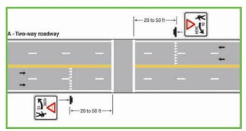
Figure 5.8. The white triangles indicate where you should stop to yield to pedestrians. The accompanying sign reminds you to be prepared to yield when pedestrians are present.
