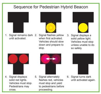
Figure 5.11. The Pedestrian Hybrid Beacon.
