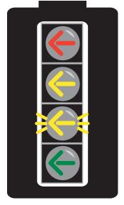
The new left-turn signal head has four signals.
